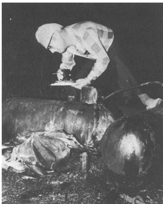
FIG. 8—Charred remains of gondola from Case 1 viewed by FAA examiner. Note structurally intact stainless steel horizontally configured propane tanks (courtesy of Albuquerque Tribune).
