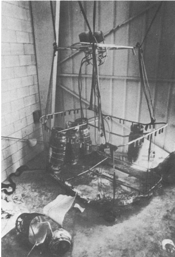
FIG. 10—Gondola remains from Case 2. Note burst aluminum propane tank (courtesy of Albuquerque Tribune).
