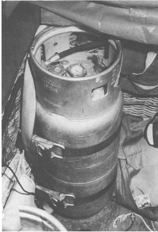
FIG. 12—Thirty-eight-litre (ten-gallon) aluminum vertically configured propane tank (photo by University of New Mexico Medical Illustrations).
